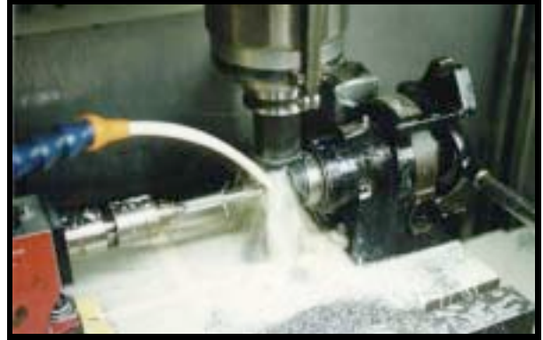
Lock spindles are precision machined on CNC Milling machines
