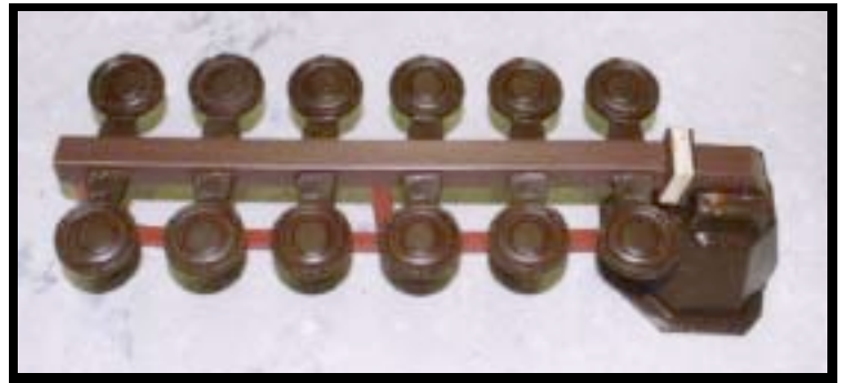
Wax Lock Escutcheons Gated & Mounted Ready for Shell Mold Application
